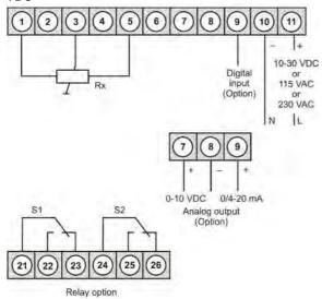
M2 with digital input and external voltage supply source
