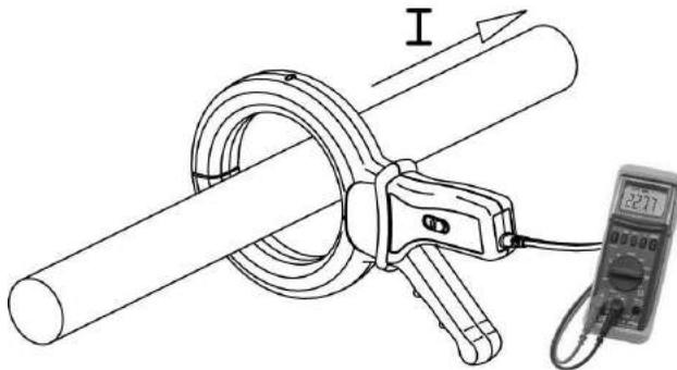
**Figure 9:** Principle for using the B102 ammeter clamp.
