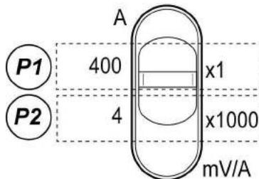
**Figure 8:** Reminder of the selector switch's positions.
