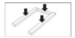
The pallet scales is designed for an even distributed load.
