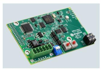
SmartLinx modules provide direct digital connection to popular industrial communications buses with true plug-and-play compatibility with products manufactured by Siemens.
