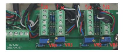
Adjustment of weighing cell J2 takes place at the potentiometer VR1. Adjustment of weighing cell J3 takes place at the potentiometer VR2. Adjustment of weighing cell J4 takes place at the potentiometer VR3. Adjustment of weighing cell J5 takes place at the potentiometer VR4. Increase the value turning to the right, reduce the value turning to the left.
