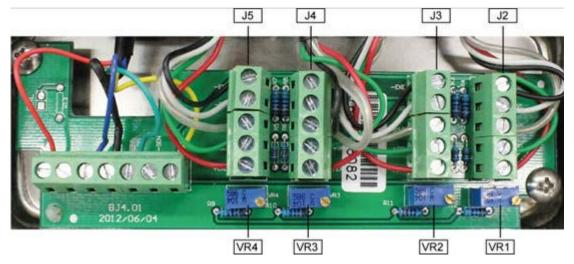
Adjustment of weighing cell 3 takes place at the potentiometer VR1. Adjustment of weighing cell 4 takes place at the potentiometer VR2. Adjustment of weighing cell 1 takes place at the potentiometer VR3. Adjustment of weighing cell 2 takes place at the potentiometer VR4. Increase the value turning to the right, reduce the value turning to the left.
