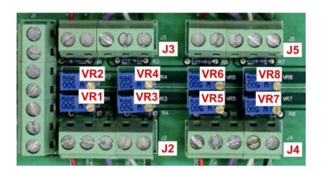
Adjustment of weighing cell J2 takes place at the potentiometer VR1 and VR2. Adjustment of weighing cell J3 takes place at the potentiometer VR3 and VR4. Adjustment of weighing cell J4 takes place at the potentiometer VR5 and VR6. Adjustment of weighing cell J5 takes place at the potentiometer VR7 and VR8. Increase the value turning to the right, reduce the value turning to the left.
