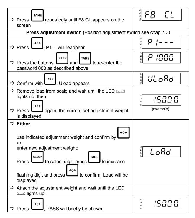
After successful adjustment the balance carries out a selftest, then it automatically returns to weighing mode.
