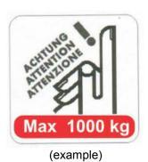
⇒ Do not exceed the nominal load of crane, crane scales or any kind of load attachment devices at the crane scales.
