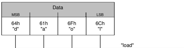
On reception of the correct signature in sub-index 1 the device restores the default parameters and then confirms the SDO transmission (initiate download response). If the restoring failed, the device responds with an Abort SDO Transfer (abort code: 0606 0000h). If a wrong signature is written, the device refuses to restore the defaults and responds with an Abort SDO Transfer (abort code: 0800 0020h). The default values are set valid after the device is reset (reset node or power cycled)
