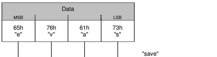
On reception of the correct signature in sub-index 1 the device stores the parameter and then confirms the SDO transmission (initiate download response). If the storing failed, the device responds with an Abort SDO Transfer (abort code: 0606 0000h). If a wrong signature is written, the device refuses to store and responds with Abort SDO Transfer (abort code: 0800 0020h).
