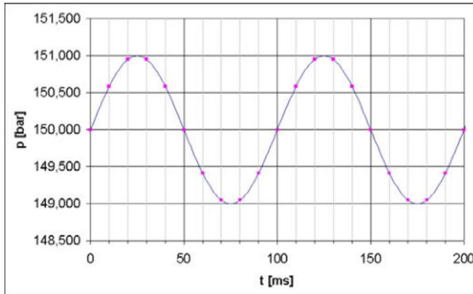
With a sample rate of 5 ms and filter value of 20, there is an averaging of the measured values of the last 100 ms.
