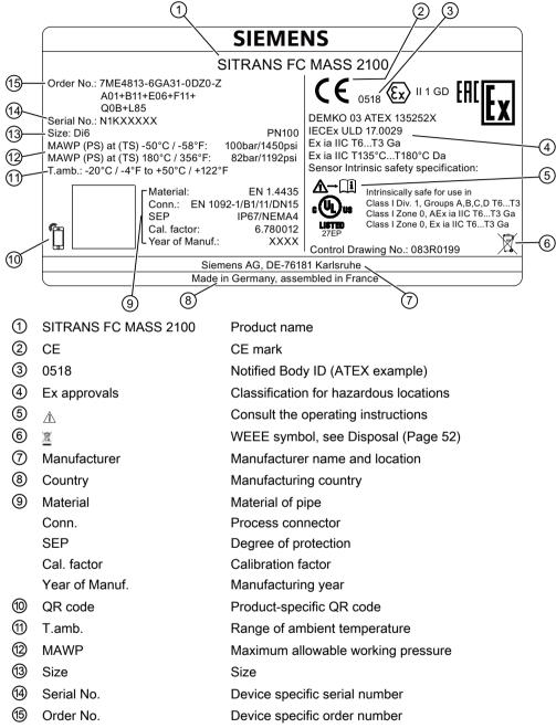
Figure 1-1 MASS 2100 nameplate example
