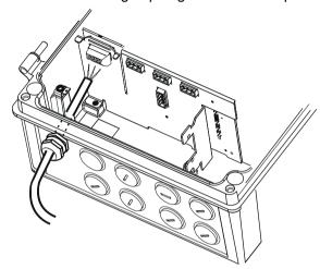
6. Restore ferrule and tighten cap to lightly hold cable in place.
