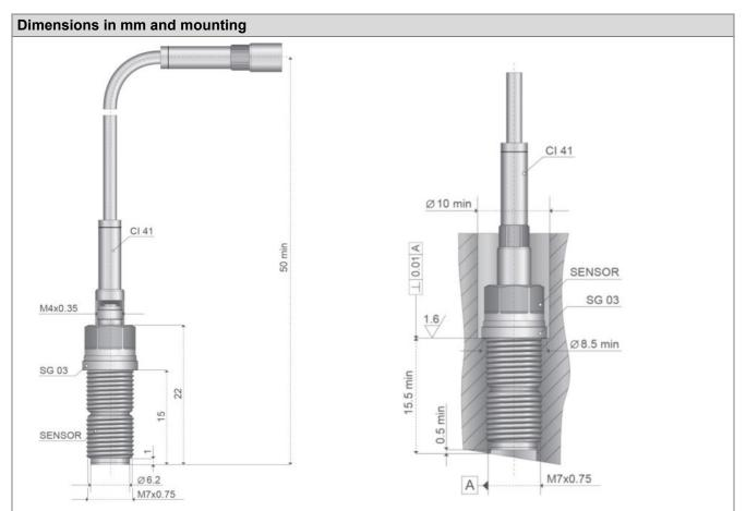
The sensor can be screwed directly into the object to be measured. The sensor rear side ( $\emptyset$  8.45 mm) seals the sensor in the mounting hole. Rapid changes in pressure are best detected when the volume in front of the membrane is kept as small as possible.
