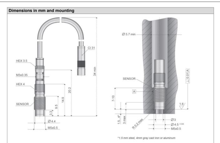
The sensor can be screwed directly into the object to be measured. The sensor front side ( $\emptyset$  4.4 mm) seals the sensor in the mounting hole. Rapid changes in pressure are best detected when the volume in front of the membrane is kept as small as possible.
