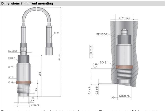
The sensor can be screwed directly into the object to be measured. The sensor rear side ( $\emptyset$  9.5 mm) seals the sensor in the mounting hole. Rapid changes in pressure are best detected when the volume in front of the membrane is kept as small as possible.
