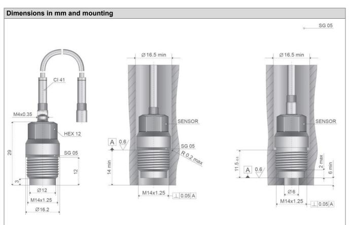
The sensor can be screwed directly into the object to be measured. The sensor rear side ( $\emptyset$  16.2 mm,  $\emptyset$  12.0 mm) seals the sensor in the mounting hole. Rapid changes in pressure are best detected when the volume in front of the membrane is kept as small as possible.
