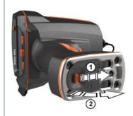
Push the battery all the way into the rechargeable battery slot until this is flush with the bottom of the handle.
