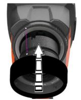
2 Align the markings on the lens and handle.
