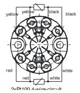
Colour coding for cable sensors (depends on type of cable e.g. Teflon-Silicone)
