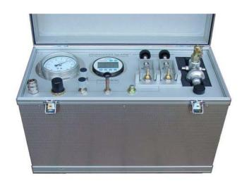
The mobile test type PRM is designed for the calibration and testing of tire pressure manometern constructed. The compressed air input flange and pressure test correspond to the filling stations and workshops occurring clutches. Equipped test is certified with a precision digital pressure gauge type HEISE fine and analog measurement Available gauge. measuring ranges of 10, 20 oder 35 bar. Allows pressure pressure next tire also brake manometer. and other pressure gauges monitored / calibrated.
