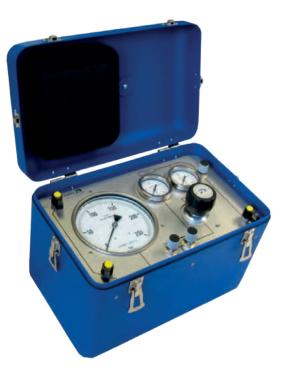
The analog pneumatic portable calibrator Model 8185 is designed for the supply and measurement of high pneumatic pressures. Model 8185 can be used for calibrating and testing high pressure transmitters, pressure switches, safety valves, etc. The built-in high pressure gas storage system makes it possible to use this test-unit at all locations, independent of any external pressure source.
