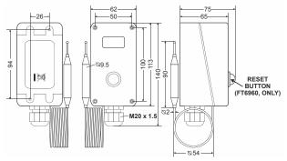
Fig. 1. Dimensions in mm
