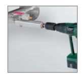
Drill under pressure with the drilling jig
