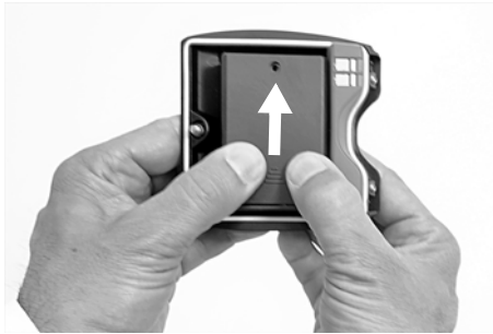
Fig. 12: Removing the cover of the battery compartment
