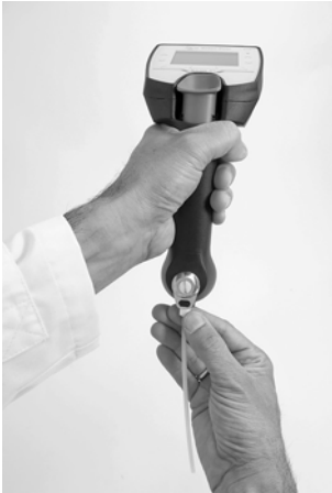
Fig. 3: Connecting the filling tube
