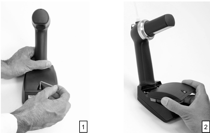
Fig. 11: Removing the battery compartment
