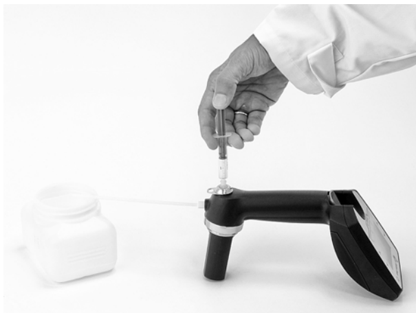
Fig. 8: Filling sample with a syringe
