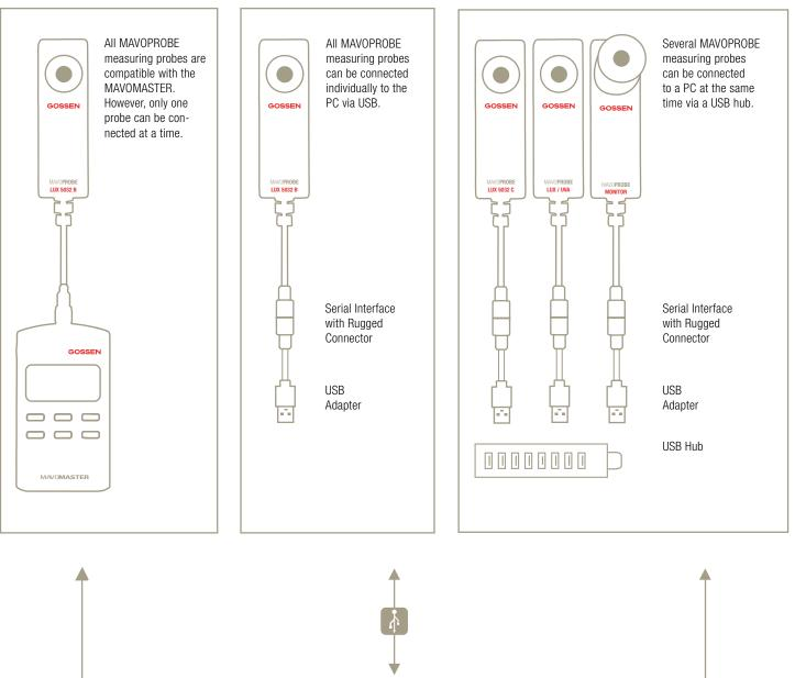
Single Channel Measuring System Multi-Channel Measuring System
