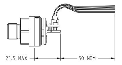
GAUGE SENSOR WITH PB PRESSURE CONNECTOR SHOWN
