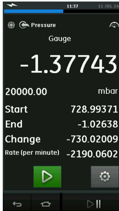
Figure 2-27 Leak Test Example
