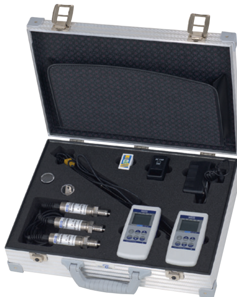
Example of a service case (temperature and pressure)
