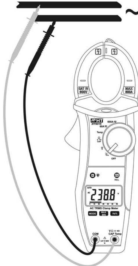
Fig. 3: Taking AC voltage measurements
