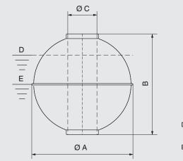
D = Limit density of the medium, immersed float volume 85 %
