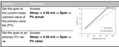
The standard value of the span after reset to defaults is 40 mm below the sealing surface of the thread connection.
