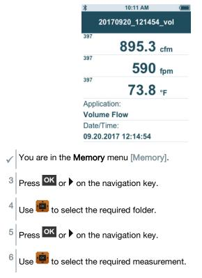
Press or b on the navigation key to display measurement results.
