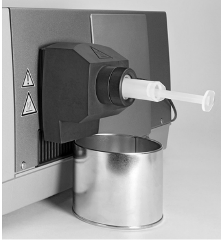
Fig. 13: Filling the sample when the syringe heating accessory is installed
