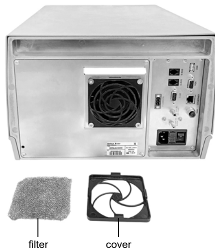
Fig. 15: Cleaning the filter of the rear fan
