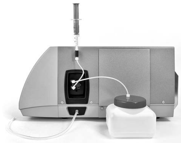
Fig. 14: Filling with a plastic syringe
