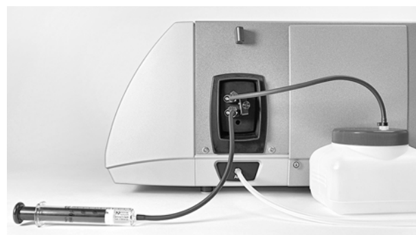
Fig. 13: Filling with a glass syringe
