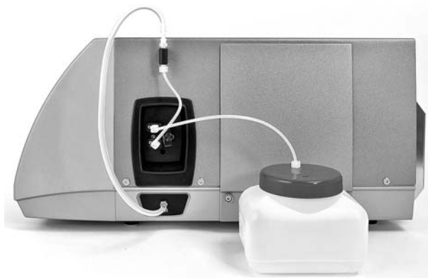
Fig. 16: Drying the measuring cells
