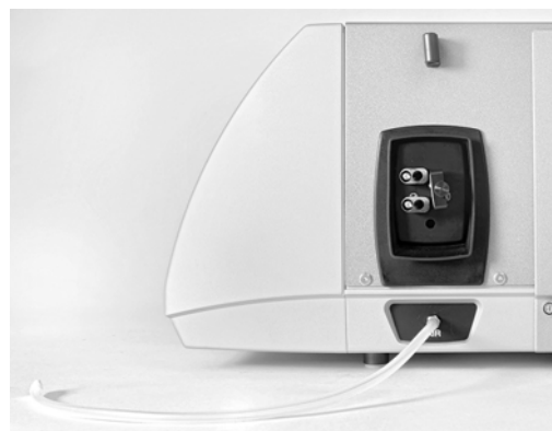
Fig. 8: Air pump hose mounted
