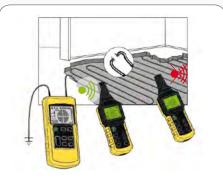
Fault detection in under-floor heating systems
