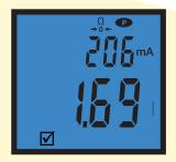
Continuity measurement at 200 mA with measurement < 2 Ω Blue screen and ✓
