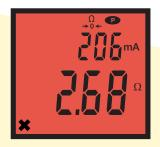
Continuity measurement at 200 mA with measurement > 2 Ω Red screen and ★
