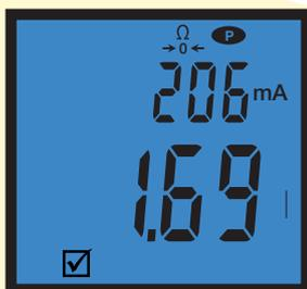
Continuity measurement at 200 mA with measurement  $< 2 \Omega$
