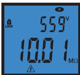
Insulation measurement in manual or locked mode or with a duration programmed using the timer
