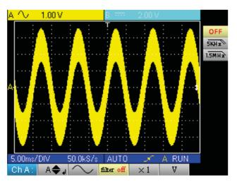
■ with the filter 5 kHz low-pass filter (the 3 MHz sinusoidal is cut):
