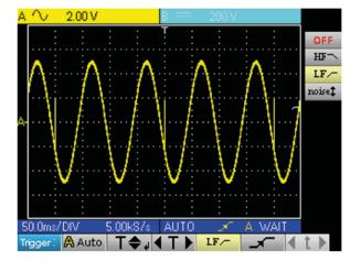
By changing the time base, the peaks can be observed correctly:
