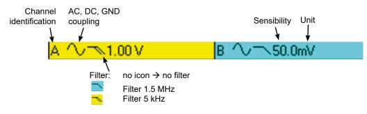
The direct data from channels A and B are displayed in this window:
