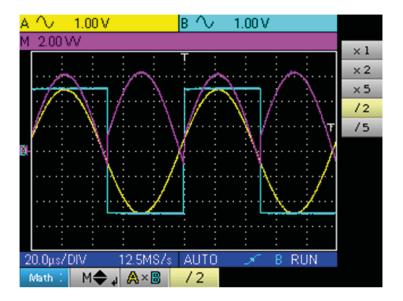
The sensitivity of channel M becomes 2 VV and the peak voltage is 3.125 \* 2 VV = 6.25 VV.
