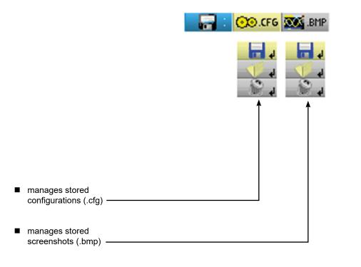
■ The .bmp file can be recovered on a PC using SX-METRO software/ Oscilloscope mode, import memory.
