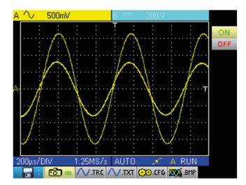
A reference memory is volatile; it is lost when the instrument is powered off, or when the channel or reference is deactivated.
