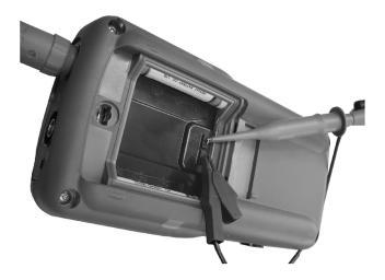
Connect the sensor to be adjusted to the calibration output under the battery housing cover, as shown opposite. Select the DC coupling for the channel to which the sensor is connected and run an autoset (icon opposite) to carry out pre-setting. Adjust the sensitivity and the vertical offset of the channel so that the signal fills the screen, and adjust the time base to 200 µs to view a signal period on the screen. Turn the BNC base of the sensor in order to access the sensor adjustment screw:
