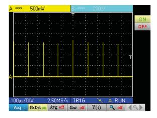
Peak detection deactivates ETS (Equivalent Time Sampling) reconstruction of a repetitive trace. Sampling is real-time for time bases  $\leq 2.5 \ \mu$ s/div.
