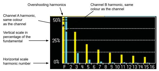
This area displays harmonics 1 to 16 of the validated channels in the form of a bar chart. The user can switch from the display of harmonics 2 to 16 to the display of harmonics 17 to 31. The max. vertical scale will depend on the zoom factor. The zoom factor can be modified using the Acq menu.
