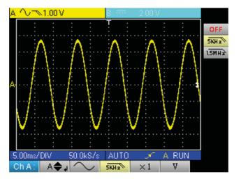
■ with the 1,5 MHz low-pass filter (the sinusoidal is partially cut):
