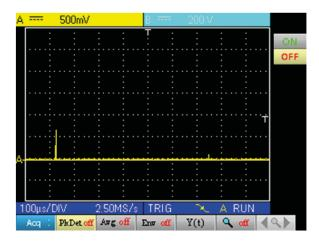
• with PkDet (the detection of the min and max obtained between two sampling steps makes it possible to view all the combs) :
