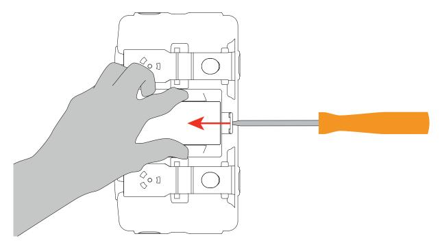
Remove the battery compartment cover, then raise the rubber plug.
