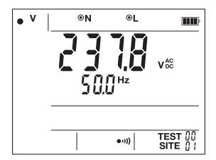
The instrument indicates whether the voltage is AC or DC.
