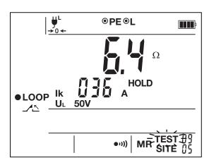
Pressing the ▶ key causes the SITE symbol to blink. You can change the site number using the ▲ key.
