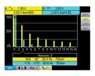
function helps to improve analysis performance and, above all, measurement when the level of a harmonic order is greater than the level of the fundamental.
