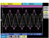
The **Autoset** of the channels is optimized for **synchronization of the signal parameters.** The waveform display can be stabilized very simply by pressing a single "magic" key.
