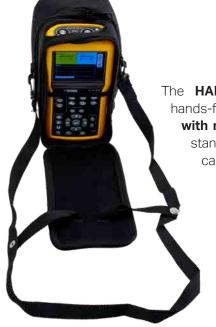
The **HANDSCOPE's** essential feature, hands-free use, is facilitated by the **bag** with **neck-strap** and the magnetized stand supplied for fastening on metal cabinets.
