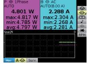
CJust as for the three instrument modes, a single press on the dedicated key gives access to the multimeter mode allowing you to measure AC, DC and AC+DC voltages and currents, resistance, continuity, capacitance, frequency, power (combination of two measurement channels), temperature (K thermocouple or infrared sensor) and motor rotation speed (optical tachometer). The instrument can also be used to test diodes and components.
