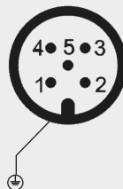
Circular connector M12 x 1, 5-pin
