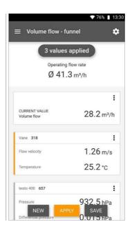
6 Apply: the current reading is applied.
