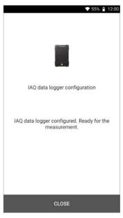
Following successful configuration, the testo 400 can be disconnected from the IAQ data logger. The measurement starts at the defined time or as soon as the setup has been completed (if the start time has been set to manual). The green LED on the IAQ data logger flashes rapidly at short intervals.
