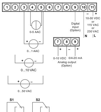
IM2 with digital input and external voltage supply source
