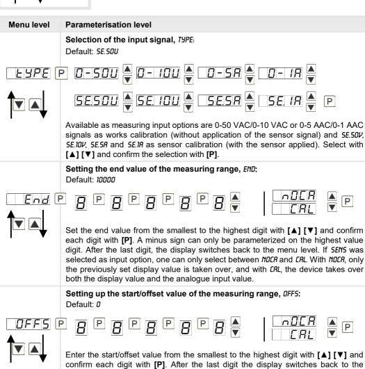
menu level. If SENS was selected as input option, one can only select between NDCR and ERL. With NDCR, only the previously set display value is taken over, and with ERL, the device takes over both the display value and the analogue input value.
