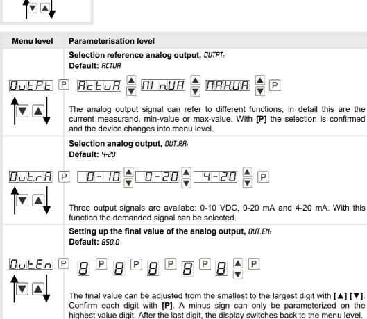
Confirm each digit with **[P]**. A minus sign can only be parameterized on th highest value digit. After the last digit, the display switches back to the menu level
