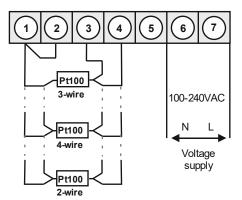
Type IM3-7TR5A.010C.770xD 2-/4-wire Type IM3-7TR5A.030C.770xD 3-wire supply of 24 VDC
