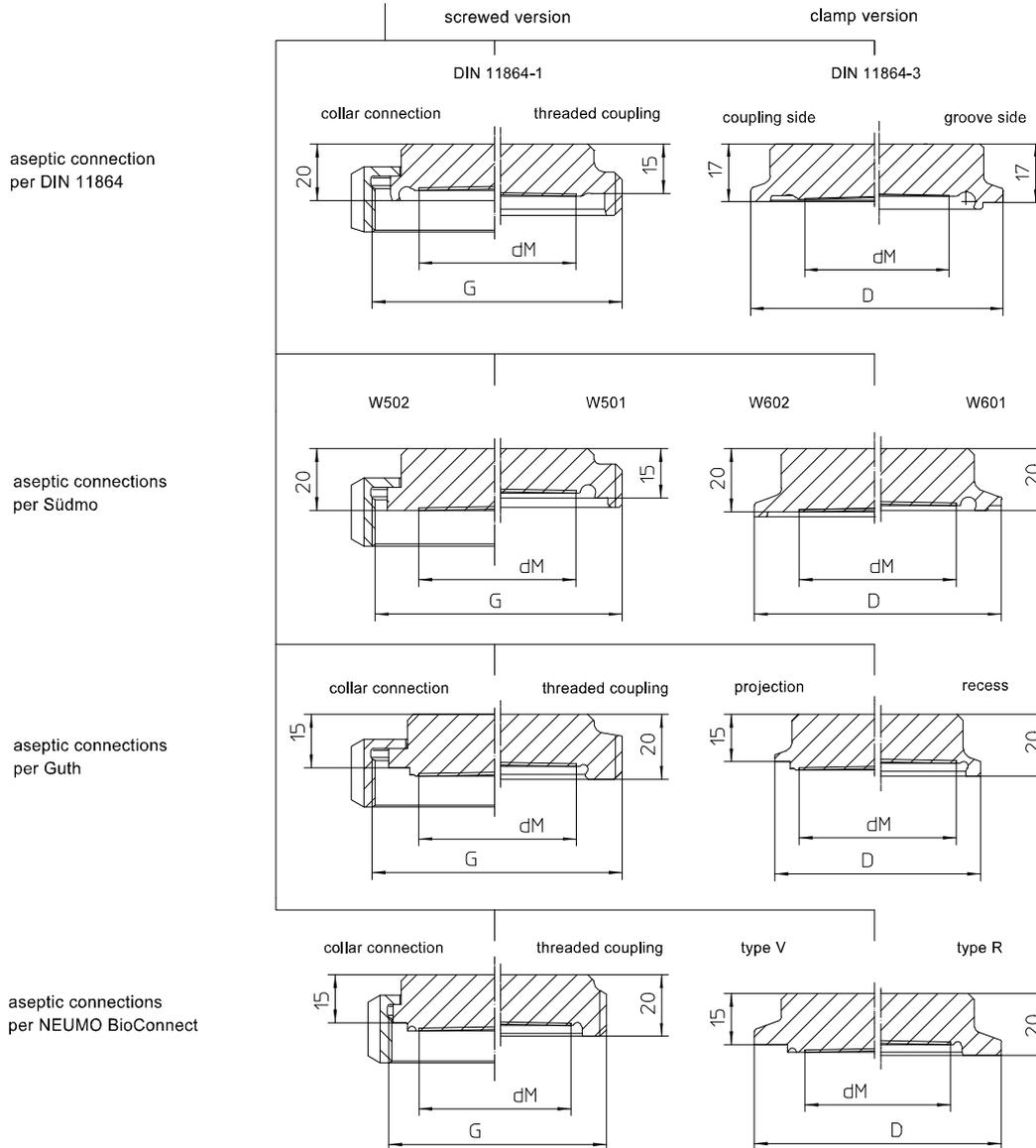
**Diaphragm seals for pipes per EN 10357 (DIN 11850) - pipe dimensions per DIN 11866 table 1 model A**
