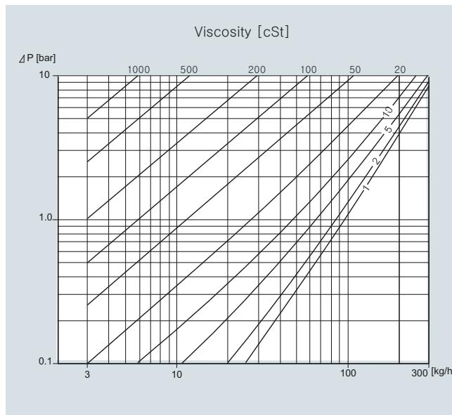
SITRANS FC300 DN 4, pressure loss, viscosity and flow rate for Hastelloy C22 / 2.4602
