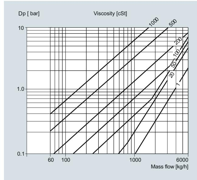
MASS 2100 DI 15 (1/2"), pressure drop for density = 101 500 kg/m<sup>3</sup>
