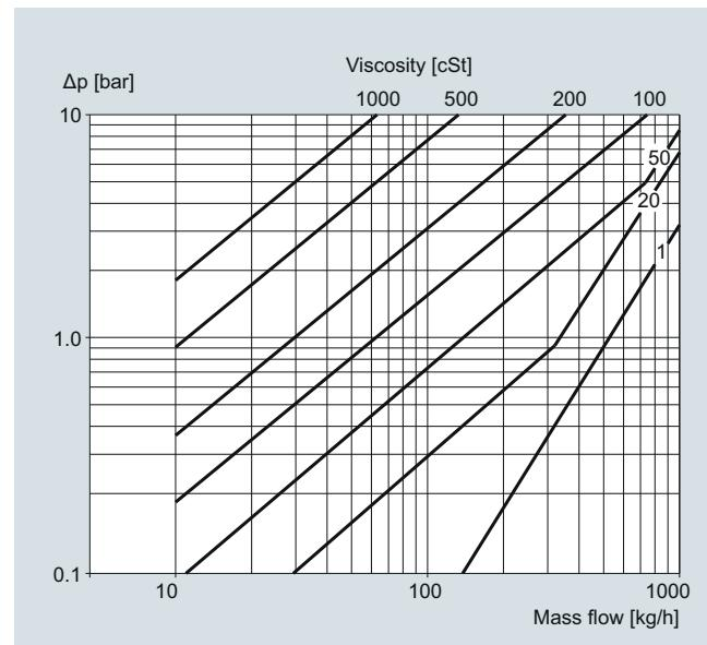
MASS 2100 DI 6 (1/4"), pressure drop for density = 1 000 kg/m<sup>3</sup>
