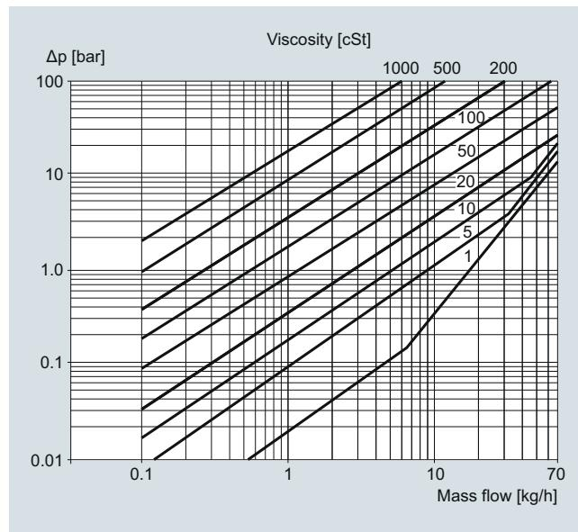
MASS 2100 DI 1.5 (1/16"), pressure drop for density = 1 000 kg/m<sup>3</sup>
