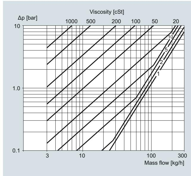
MASS 2100 DI 3 (1/8"), pressure drop for density = 1 000 kg/m<sup>3</sup>
