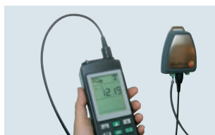
Inspection of transmitters with 4 to 20 mA interface
