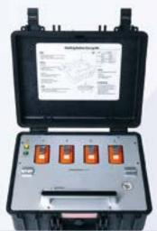
Bump testing portable monitors is becoming more and more prevalent in the market. Ensuring sensors are responding to a known concentration of gas remains the best way to verify the monitor is working as intended and has not become impeded.
