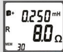
Screen 3: Value of the resistive and inductive part of the impedance measured
