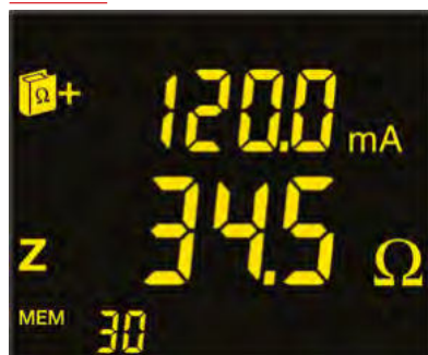
Screen 1: Impedance and leakage current
