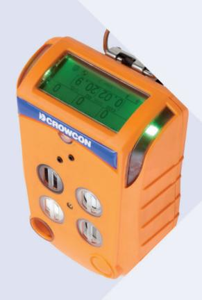
Gas-Pro is compatible with a wide range of sensor options including an Infrared (IR) sensor for detection of flammable gasses and CO2 with guaranteed fast response, very low maintenance requirements, long lifespan and fail-safe operation. In addition Gas-Pro is also available with a PID sensor for detection of a wide range of VOCs perfect for the chemical industry especially if working with tanks containing solvents.
