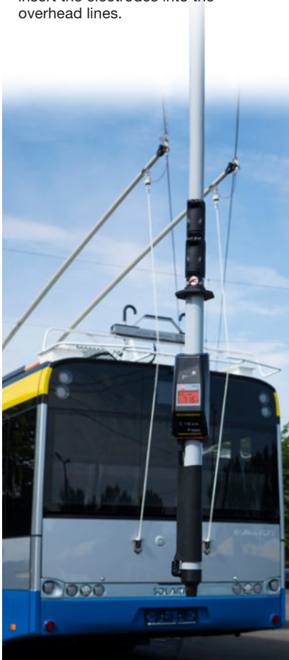
Clear indication of voltage by LCD, LED and acoustic signal.
