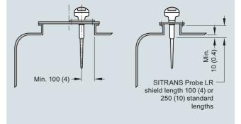
SITRANS Probe LR installation, dimensions in mm (inch)
