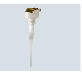
SITRANS Probe LR is a 2-wire, 6 GHz pulse radar level transmitter for continuous monitoring of liquids and slurries in storage vessels with nominal pressure and temperature, to a range of 20 m (66 ft).
