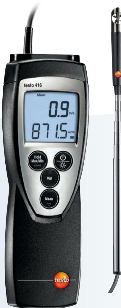
The testo 416 is a compact anemometer with a fixed vane probe. The measuring instrument is particularly suitable for flow velocity measurements in ducts thanks to the extendable telescope (max. length 890 mm, diameter 16 mm). The volume flow is directly shown in the display. For volume flow calculation purposes, the duct cross-section area can be conveniently entered into the testo 416. The timed and point mean value calculations provide information on the average volume flow.
